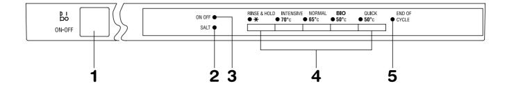
In this fully integrated appliance the controls are located on the top of the door. When selecting a programme, the door needs to be open.
